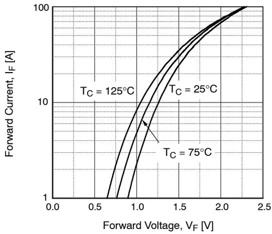
**Figure 3. Typical Forward Voltage Drop vs. Forward Current**
