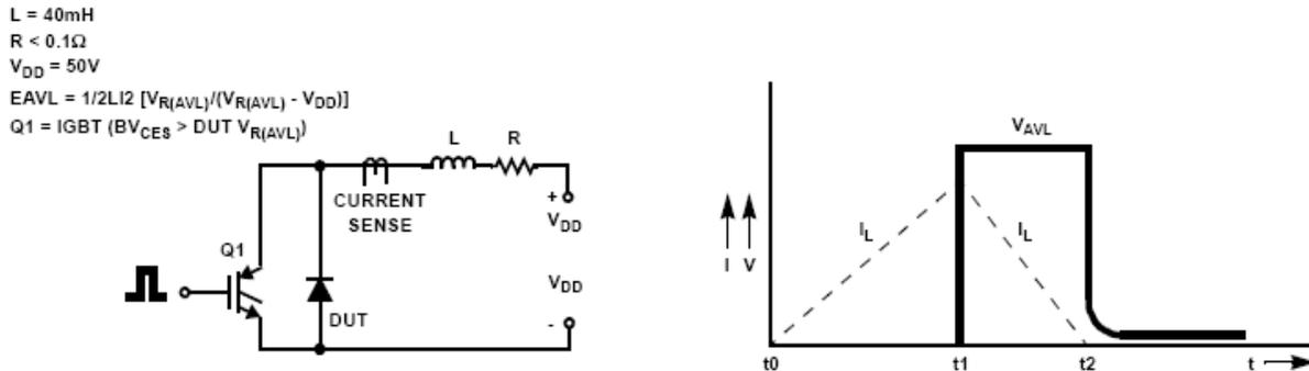
Figure 2. Unclamped Inductive Switching Test Circuit & Waveform
